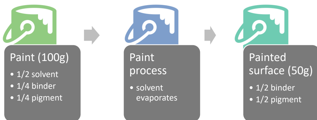
Figure 17. Illustration of the Changes to Mass and Ratio after the Evaporation of a Solvent
