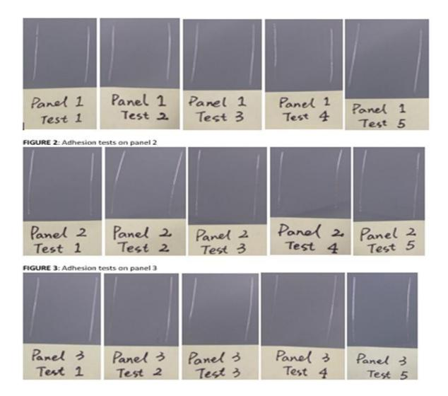
Figure 3. Adhesion Test Panels with Duplex TCP & Hot Water Seal
