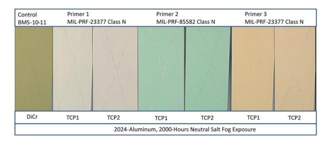
Figure 4. Scribed Corrosion Resistance, Type IIB, TFSAA, ASTM B 117 Controlled Neutral Salt Fog, (NSF)
