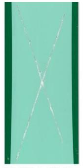
TSAA w/TCP System 1 & Hot DI Water seal; water based nonchromated primer.
