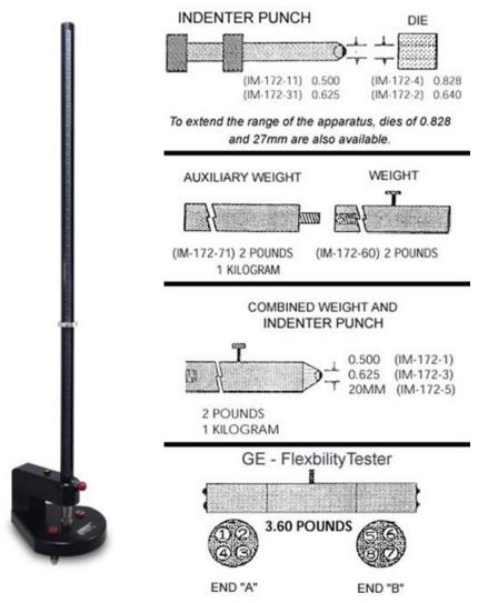
Figure 11. ASTM D 6905 Test Apparatus
