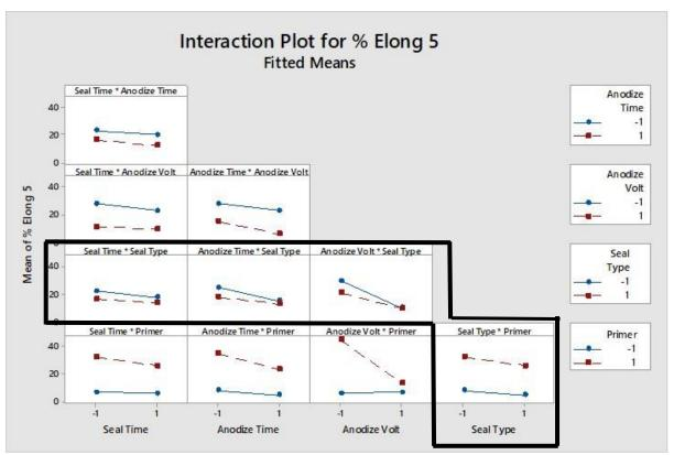
Figure 14. Process Factor Interactions, Organic Finish Flexibility, 5-Vol% TCP
