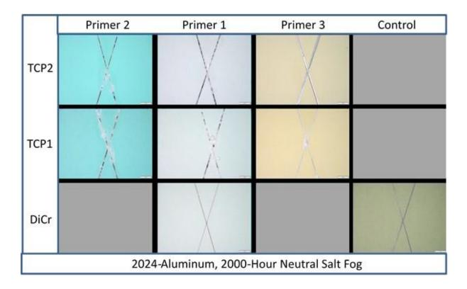
Figure 5. Scribed Corrosion Resistance, Corrosion Product in Scribe, Type IIB, 2000-Hours NSF
