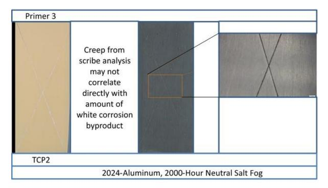
Figure 7. Evaluation of Corrosion Creep Beyond Scribe, (Primer Removed), Type IIB, 2000-Hours NSF
