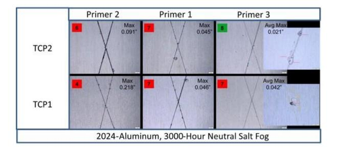
Figure 8. Evaluation of Corrosion Creep Beyond Scribe, Type IIB, 3000-Hours NSF
