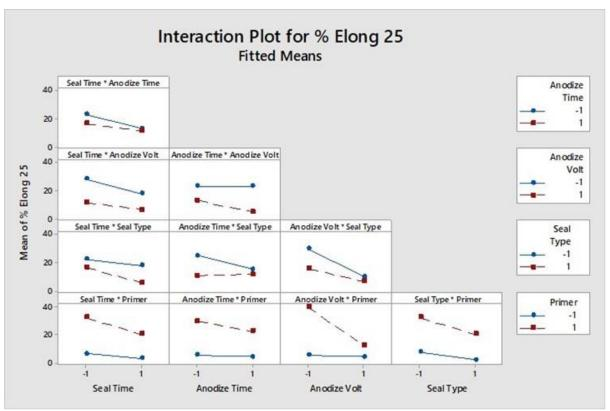
Figure 17. Process Factor Interaction, Organic Finish Flexibility, 25-Vol% TCP
