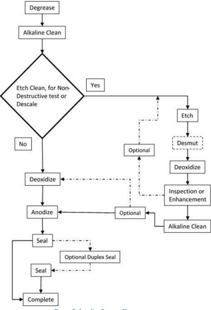
Figure 2. Anodize Process Flow
