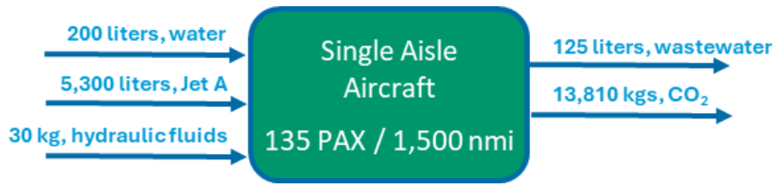
Figure 5. Example of the reference flow and its inputs and outputs for a functional unit of "to transport 135 passengers 1500 nmi"
