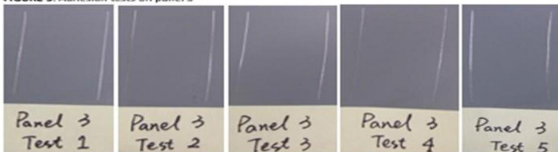
Figure 3. Adhesion Test Panels with Duplex TCP & Hot Water Seal
